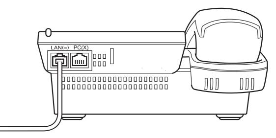
**Note:** The PC connector on the IP terminal is exclusively for a PC connection, not a second IP terminal.
